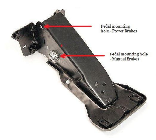
The Ford factory brake pedal support contains two mounting positions for both the original manual brake pedal and the power brake pedal. The new power brake pedal will mount in the upper hole located closest to the firewall. This position ensures proper leverage to actuate your brake system with comfortable pedal pressure.
